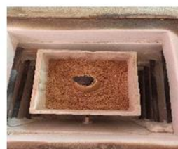
Fig. 9: Placing of Kupi in V.M.F.
