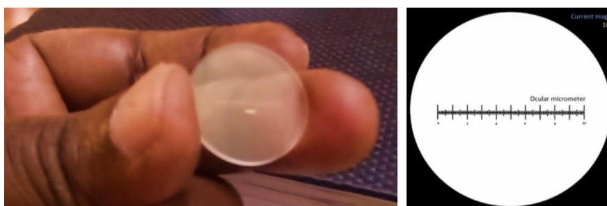
Figure 1: Showing Ocular Micrometer (OM) with 10 non-standard divisions etched at centre.
