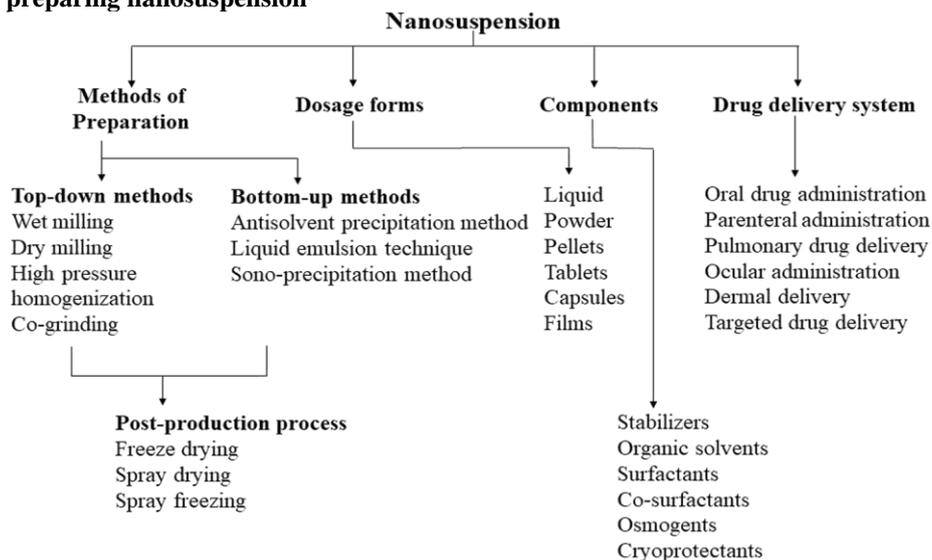
**A. High-pressure homogenization<sup>[7]</sup>** This method is based on cavitation process. The suspension containing a drug and surfactant is forced under pressure through a nanosized aperture valve of a high-pressure homogenizer.
