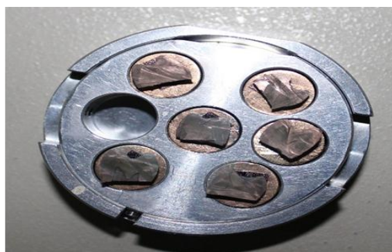
Fig 1: Gold sputtered samples in SEM stub.
