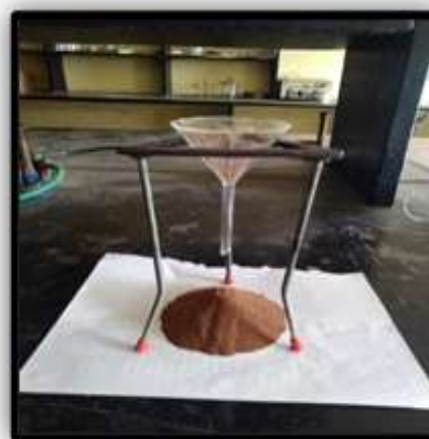
Fig: Angle of repose.
