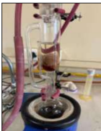
Figure 5: Soxhlet extraction of Cinnamaldehyde.
