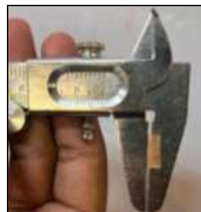
Figure 16: vernier calliper showing thickness of film.
