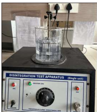
Figure 19: Basket showing disintegration of film.
