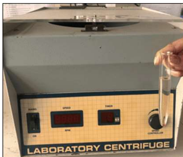
Figure 24: Centrifugation for glucose adsorption assay.
