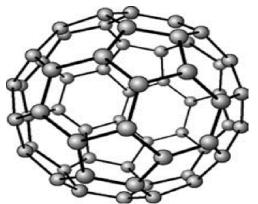
Fig no.5: Schematic representation of fullerenes.
