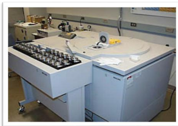
Figure no 02 and 03: Showing XRF spectrometer with the sample port on top and a set of samples in silver metallic holders in the sample changer in front.
