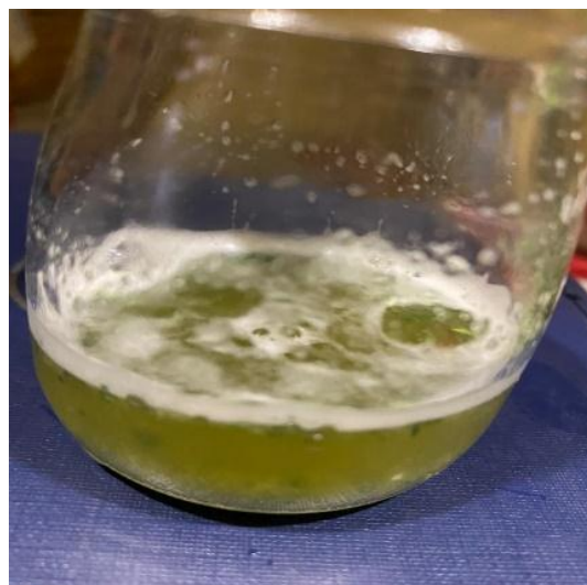
Fig. 1: Foam obtained with raw potato paste and curry leaves paste mixed in water. ( After peeling the skin raw potato pieces were grated and then grinded with 10ml water to obtain potato paste, Sixty .fresh curry leaves were grinded with 10ml water to get curry leaves paste. To this a few drops of vegetable oil like palm oil can be added as lubricant.
