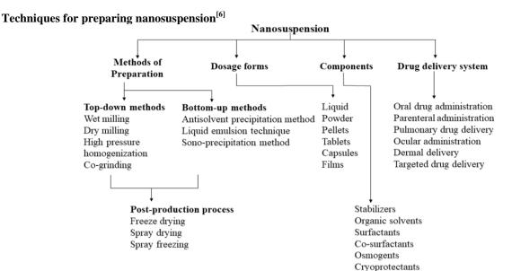
**A. High-pressure homogenization**<sup>[7]</sup> This method is based on cavitation process. The suspension containing a drug and surfactant is forced under pressure through a nanosized aperture valve of a high-pressure homogenizer.
