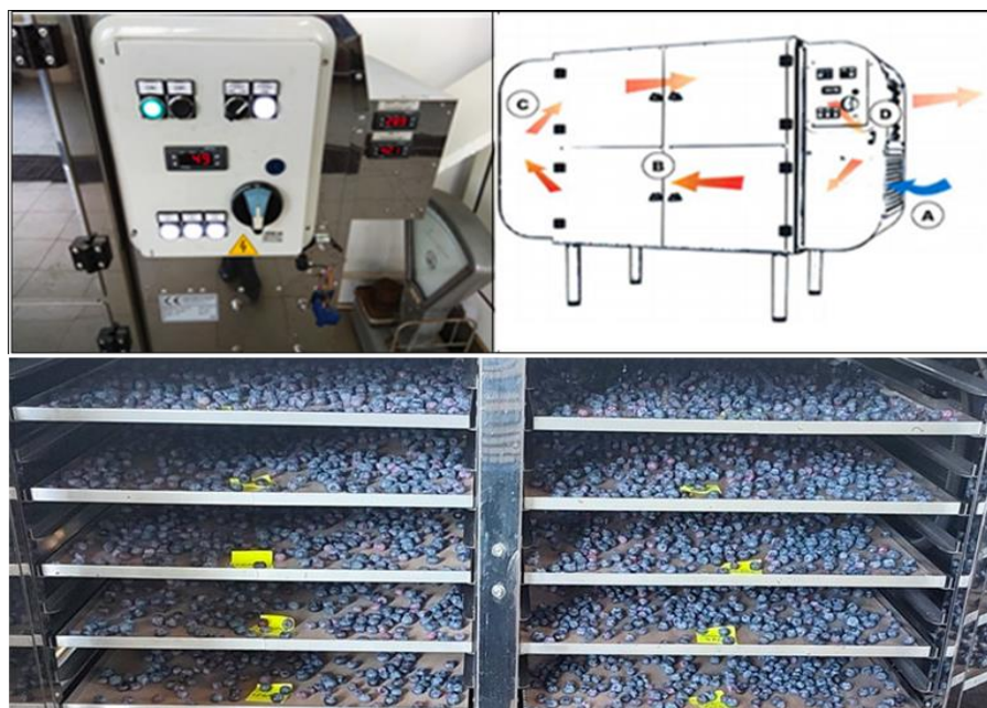
Figure 2: Convective dehydration process of organic blueberries inside the dryer.
