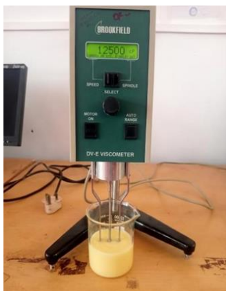
Fig 2: Viscosity Measurement by using Brookfeild.
