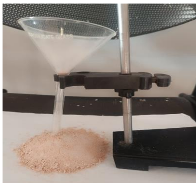
Fig no. 6: Angle of repose.
