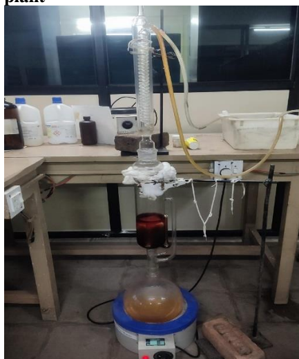
Plate 3 - Photograph showing Soxhlet's apparatus for hot continuous extraction
