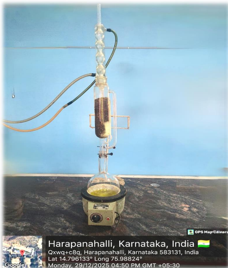
Figure 3: Soxhlet Extraction of Cordia dichotoma G. Forst leaves.
